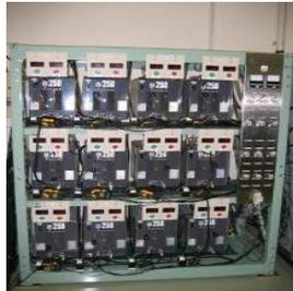
Fig. 3 Setup of the twelve-phase AC power supply
