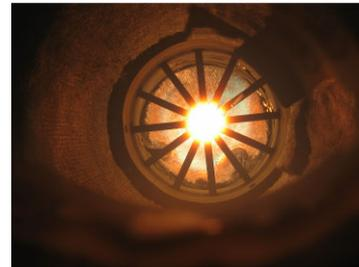
Fig. 4 Photograph of the twelve-phase AC arc discharge
