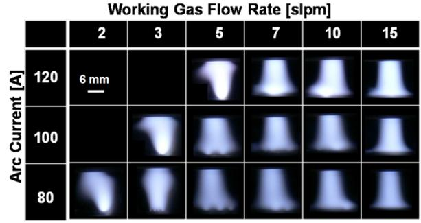
Fig. 3 CCD camera images of arc appearance modes for different arc current and the working gas flow rate.
