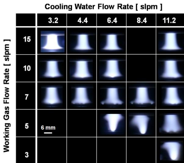
Fig. 5 CCD camera images of the arc appearance modes for different working gas flow rate and cooling water flow rate with constant arc current: 100 A.
