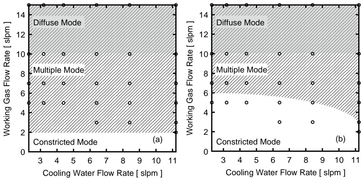
Fig. 8 The comparison between the arc-anode attachment mode (a) before evaporation and (b) after evaporation, as a function of flow rate of working gas and cooling water flow rate with 100 A of arc current.
