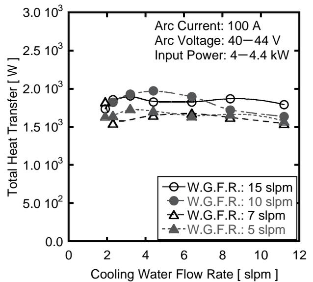
Fig. 6 The relationship between the cooling water flow rate and the total heat transfer for different working gas flow rate.
