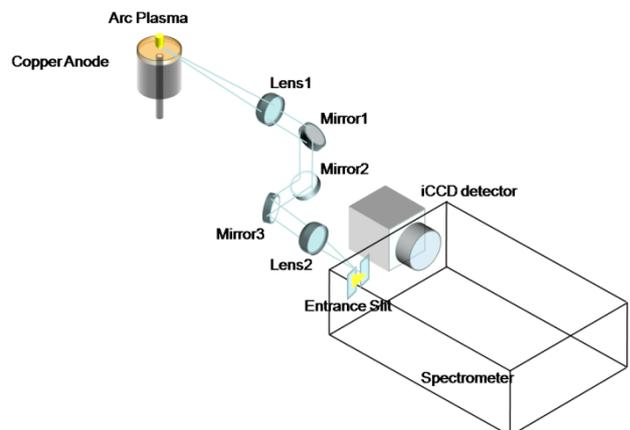
Fig. 2 The schematic of the spectroscopic system.
