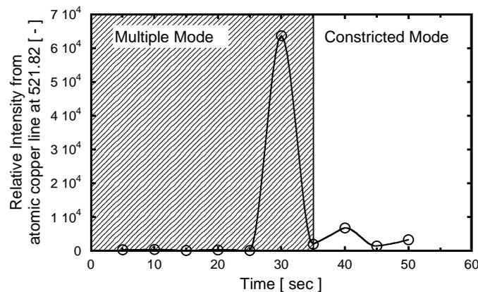
Fig. 7 The emission intensity at 521.82 nm from copper vapor as a function of time, at 100 A of arc current, 5 slpm of working gas flow rate and 8.6 slpm of cooling water flow rate. Different modes are characterized as follows. Shaded area: multiple mode. White area: constricted mode.
