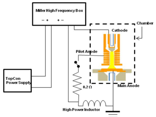
Fig. 1 Electrical schematic of the experimental setup.
