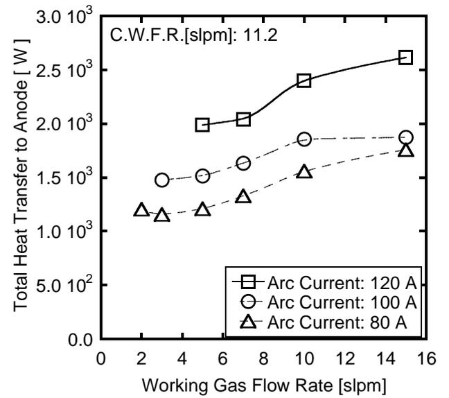
Fig. 4 The relationship between the working gas flow rate and the total heat transfer for different arc current.
