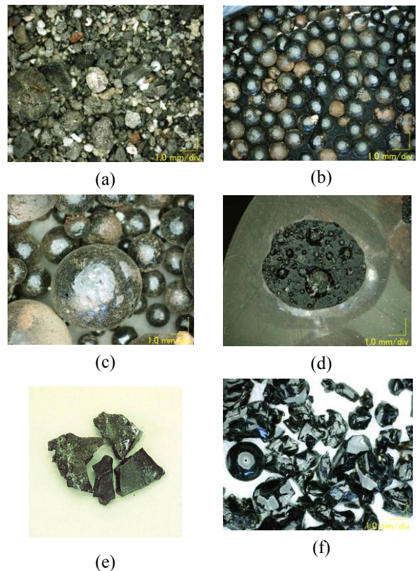
Fig.8 Photographs of incineration ashes; (a) before melting, (b) melted (primary treatment), (c) melted (secondary treatment), (d) cross section image, (e) cullet-like, (f) water crashed
