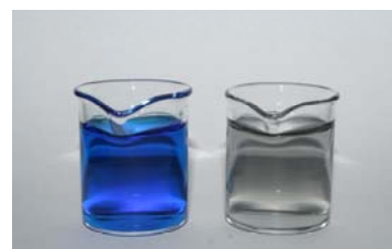
Figure 3. A comparison between untreated (left) and plasma treated (right) methylene blue solution
