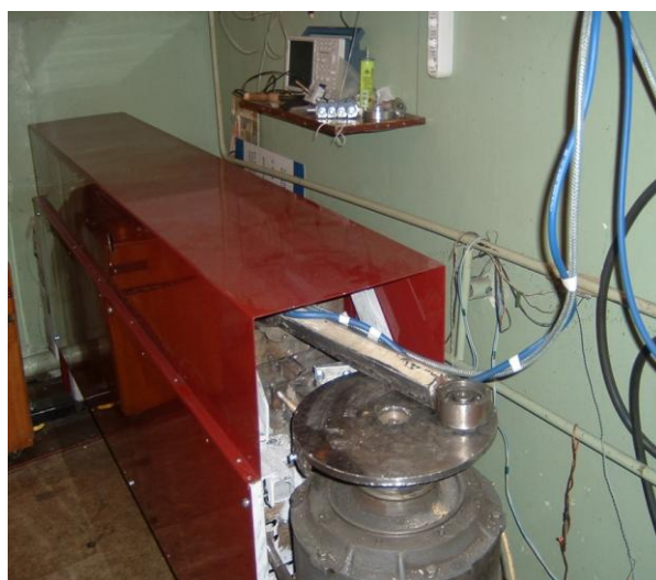
Fig.1 The appearance of the reactor. In the foreground is the engine with a crank mechanism and tension rods
