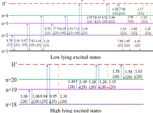
Fig. 8 Flows of electrons for low lying excited states and high lying excited states ( \text{m}^{-3}\text{s}^{-1} ). The straight arrows denote the non-radiative processes and the dashed arrows represent the radiative processes. The brackets denote the power of 10 by which the number should be multiplied ( t=1.0 \times 10^{-6} s).
