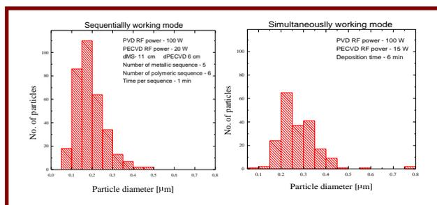
Figure 4. Histogram of particles distribution for the Cu-polysiloxane composite obtained in sequential and simultaneous working modes
