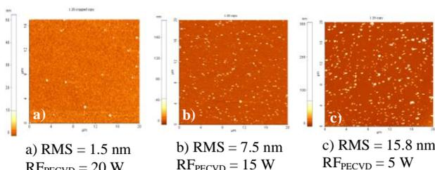
Figure 3. AFM images of the Cu-HMDSO composites synthesized in simultaneous mode as a function applied RF power on the PECVD plasma source (RF on PVD = 100 W).
