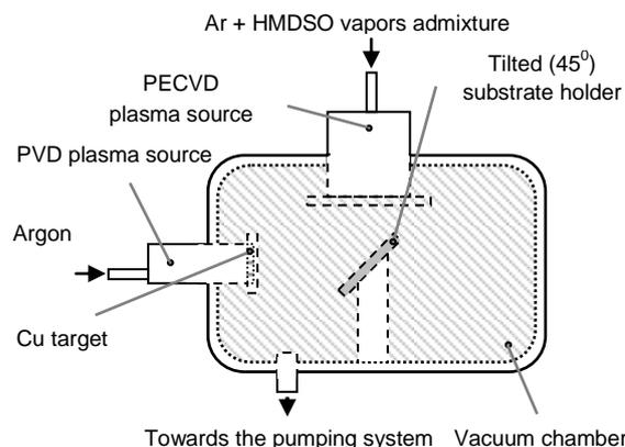
Figure 1. Schematic of the experimental set-up for the synthesis of Cu-polysiloxane composites
