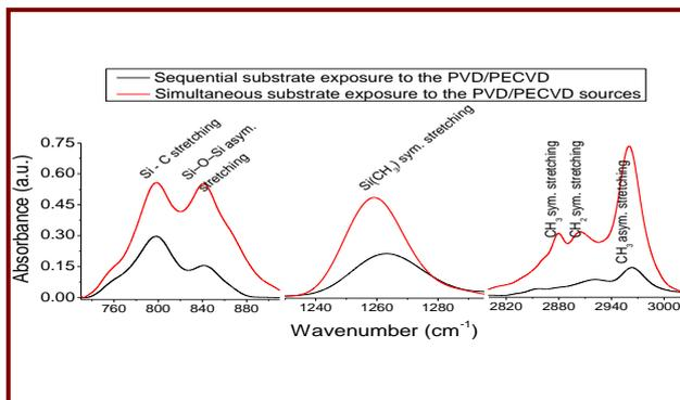
Figure 6. Comparison of the FTIR spectra of Cu-polysiloxane composites obtained in sequential (black) and simultaneous (red) working modes.
