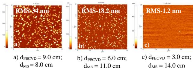
Figure 2. AFM images of the Cu-HMDSO composites synthesized in sequential mode as a function of distance from the PECVD (20 W) and PVD (100 W) plasma source
