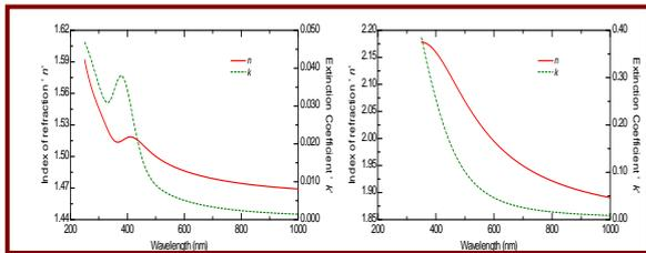
Figure 5. Comparison of the optical constants ( $n$ ,  $k$ ) of the Cu-polysiloxane with different metallic exposure time: 10 s (left); 60 s (right); exposure time for HMDSO was 60 s in all cases.
