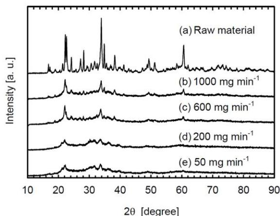
Fig.2 XRD patterns of raw  $\text{Li}_4\text{SiO}_4$  powder and products according to powder feeding rate at 5 L/min argon flow rates for carrier and additional sheath gases.
