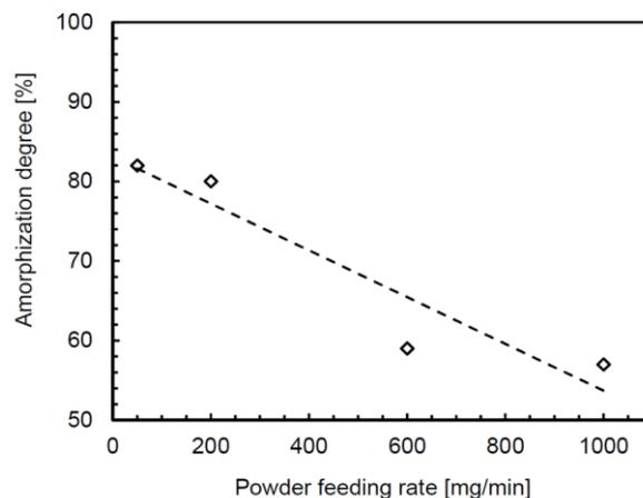
Fig.3 Amorphization degree of  $\text{Li}_4\text{SiO}_4$  according to powder feeding rate at 5 L/min argon flow rates for carrier and additional sheath gases.
