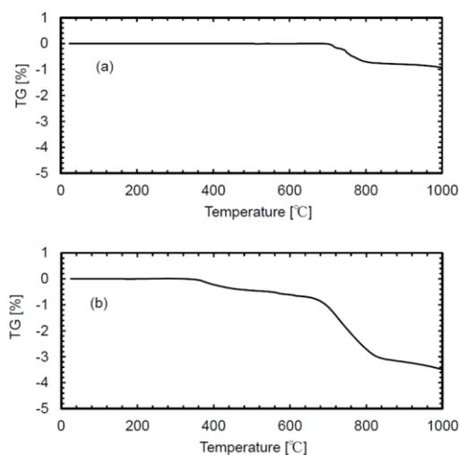
Fig.8 TGA results on amorphous  $\text{Li}_4\text{SiO}_4$  nanoparticles to for (a) 2 hours and (b) 2 months after synthesized at 200 mg/min for raw powder feeding rate.
