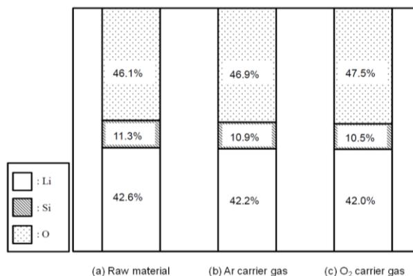
Fig.9 XPS results on (a) raw material and amorphous  $\text{Li}_4\text{SiO}_4$  nanoparticles after RF thermal plasma treatment with (b) Ar carrier gas and (c)  $\text{O}_2$  carrier gas at 200 mg/min for raw powder feeding rate.
