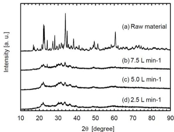
Fig.5 XRD patterns of raw  $\text{Li}_4\text{SiO}_4$  powder and products according to the flow rate of argon carrier gas at the fixed powder feeding rate of  $200\ \text{mg}/\text{min}$ .
