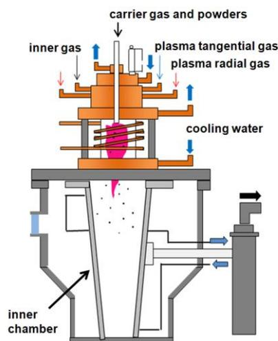
Fig.1 Schematic diagram of RF thermal plasma system for the synthesis of amorphous  $\text{Li}_4\text{SiO}_4$  nanoparticles.
