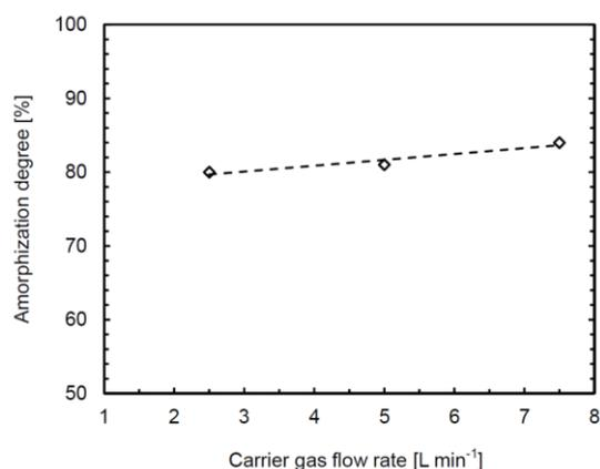
Fig.6 Amorphization degree of  $\text{Li}_4\text{SiO}_4$  according to the flow rate of argon carrier gas at the fixed powder feeding rate of  $200\ \text{mg}/\text{min}$ .
