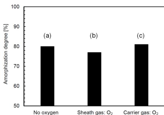
Fig.7 Comparison of amorphization degrees of  $\text{Li}_4\text{SiO}_4$  with different working gas conditions of (a) pure argon, (b) oxygen additional sheath gas, and (c) oxygen carrier gas at 200 mg/min for powder feeding rate.
