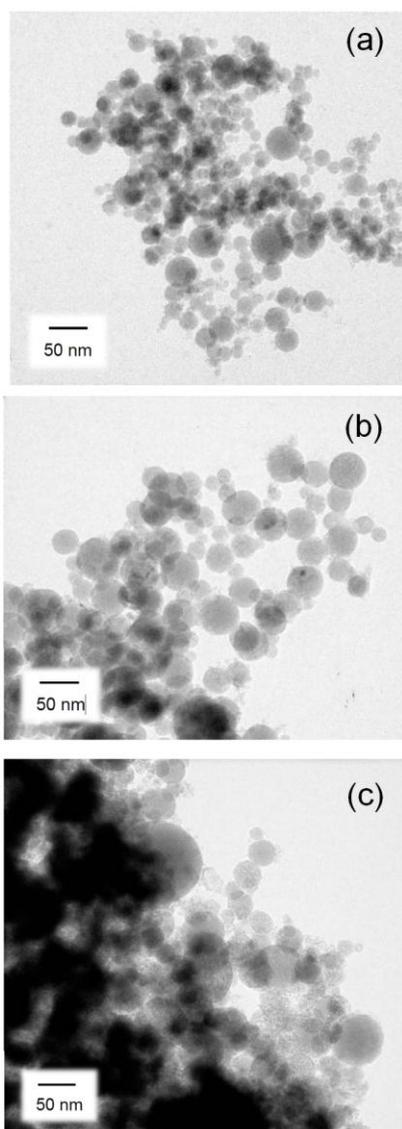
Fig.4 TEM images of synthesized amorphized  $\text{Li}_4\text{SiO}_4$  nanoparticles in different powder feeding rates of (a)  $200\ \text{mg}/\text{min}$ , (b)  $600\ \text{mg}/\text{min}$ , and (c)  $1000\ \text{mg}/\text{min}$  at  $5\ \text{L}/\text{min}$  argon flow rates for carrier and additional sheath gases.
