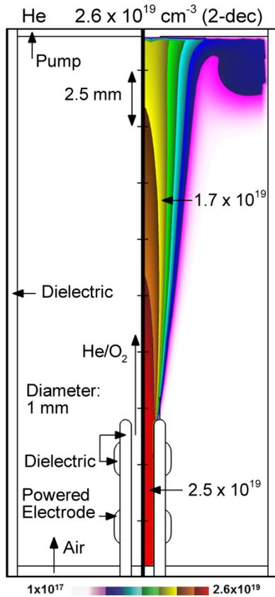
Fig. 1. (Left) Schematic of 1 mm inner diameter plasma jet. (Right) The density of helium shows the steady state flow.
