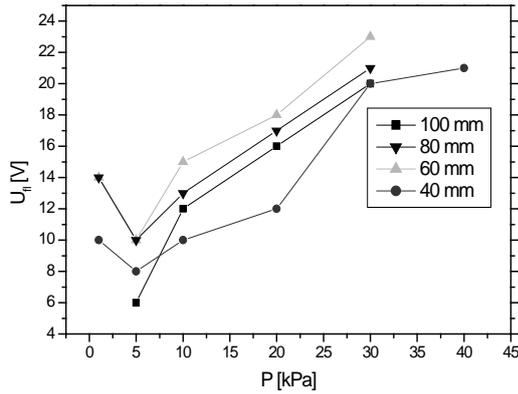
Fig. 3. Dependences of floating potential at jet centerline on pressure at several distances from the torch nozzle exit.
