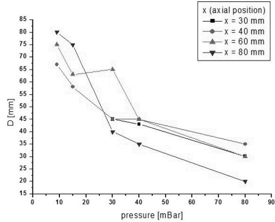
Fig. 6. The diameters of conduction area in dependence on pressure for several distances  $x$  from the torch nozzle exit.
