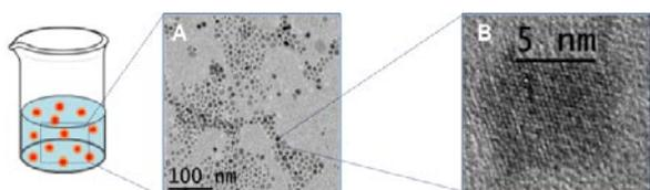
Fig. 2. TEM analysis of 3 weight% of ZnO in HMDSO. A: 25 000X magnification, B: 500 000X magnification.
