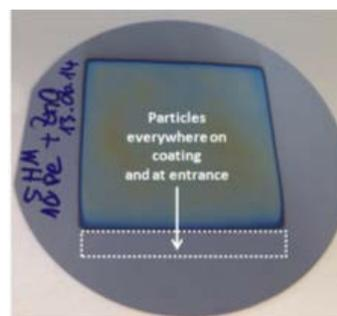
Fig. 5. Example of a silica coating with ZnO NPs
