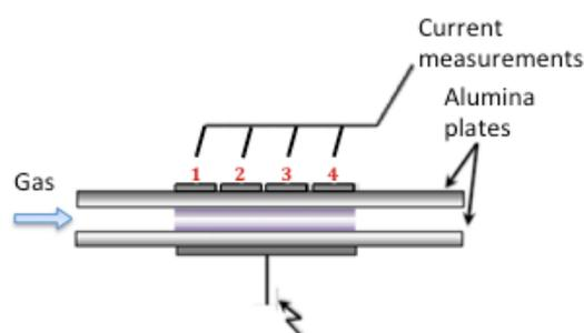
Fig. 1. Schematic of the split electrode.
