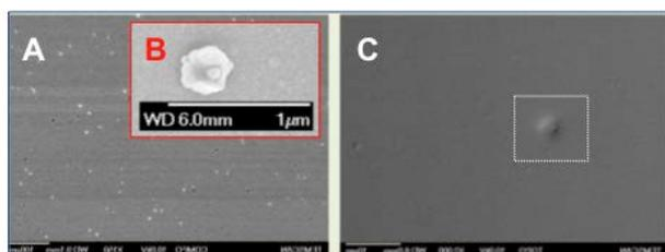
Fig. 6. SEM analysis. SEM analysis. A: ZnO particle distribution inside SiOx matrix (backscattering mode) B: Agglomerate on the surface C: Topography image of embedded ZnO particle inside SiOx matrix
