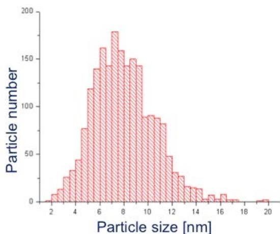
Fig. 3. Size distribution of ZnO particles in HMDSO calculated from TEM analysis.
