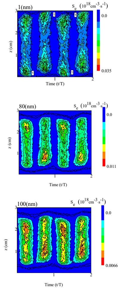
Fig.5. Spatiotemporal plots of electron impact source term during two rf cycles in  $\text{SiH}_4$  discharge driven by 50 MHz power supply, for different dust particles radius in the plasma. First row: 1 nm, second row: 80 nm, third row: 100 nm. The reversal electric field heating mode are labeled “1” in the graphs.
