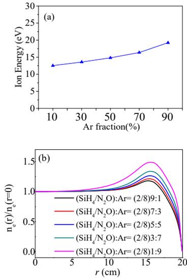
Fig.4. The ion bombardment energy on the electrode as the function of Ar fraction in the mixture gas (a) and the radial distributions of electron density at the center of discharge for different Ar fraction in the mixture gas (b) at the pressure of 266 Pa. Other discharge conditions are same as in Fig. 3
