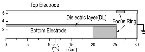
Fig.1. Schematic diagram of the cylindrical CCP reactor taken into consideration in SiH<sub>4</sub>/N<sub>2</sub>/O<sub>2</sub> discharge
