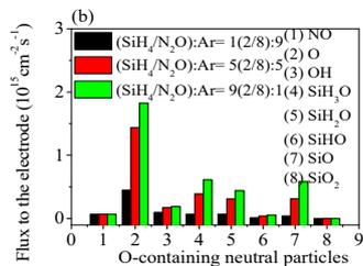
Fig. 3 Fluxes of the neutral particles containing Si (a) and O (b) on the powered electrode with different Ar fraction in the mixture gas of SiH<sub>4</sub>/N<sub>2</sub>O/Ar. The discharge condition is as follow: 13.56 MHz, 70 V power supply and 40 Pa pressure
