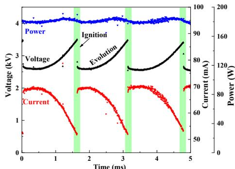
Fig. 2 Waveforms of discharge voltage, current and power
