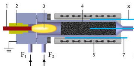
Fig. 1 Schematic diagram of the PCR reactor
