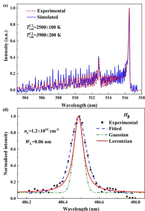
Fig. 3 Simulated and measured spectra of (a) C2 and (b)  $\text{H}_\beta$  at discharge power of 180 W and a gas mixture of  $\text{CH}_4/\text{CO}_2/\text{H}_2\text{O}$
