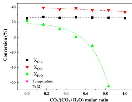
Fig. 4 Effect of  $\text{CO}_2/(\text{CO}_2+\text{H}_2\text{O})$  molar ratio on conversions and outlet temperature of GA reactor
