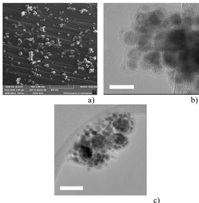
Fig.2 SEM and HRTEM pictures of Cu/nylon like NPs.
