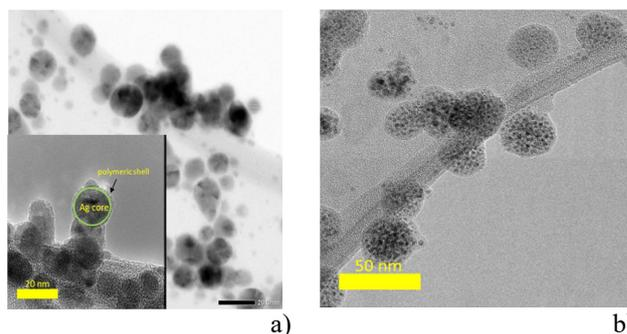
Fig 1. HRTEM of the samples prepared at 1 % (a) and 4% of HMDSO in the working gas mixture.
