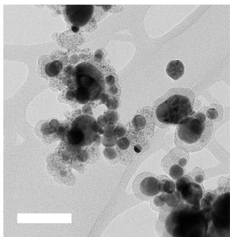
Fig.3. An example of HRTEM micrograph of nylon like NPs coated by silver.
