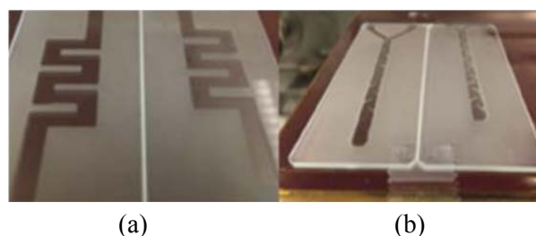
Fig. 3. Top and bottom of the two designs from Figure 2. For clarity the hydrophilic tracks are visualized with steam.
