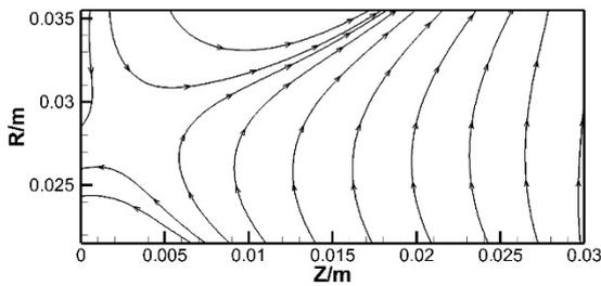
Fig. 1. Magnetic field configuration and simulation area of Hall thruster
