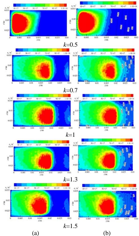
Fig. 2. Spatial distribution of electron density, ion density and equipotential lines with different  $k$ . (a) electron density; (b) ion density and equipotential lines
