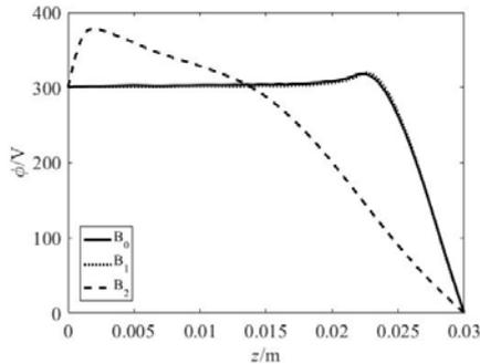
Fig. 4. Axial distribution of potential with different magnetic field configuration
