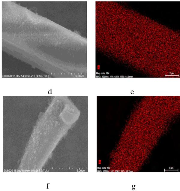
Fig.1 SEM and TEM images of phosphor powders and the distribution of the Al o phosphor; b-TEM image of uncoated powder (the scale bar is 50 nm); c- TEM image of 500 cycles of ALD  $\text{Al}_2\text{O}_3$  coating powders (the scale bar is 50 nm); d-SEM image of coated phosphor powder before immersed in water; e-EDX mapping of Al in (d); f- SEM image of coated phosphor after soaked in water for 24 hours; g- EDX mapping of Al in (f)n the surfaces (a- SEM images of uncoated .
