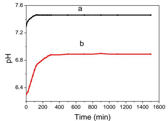
FIG.2 The variation of pH values versus immersing period. (a) uncoated powder; (b) 500 cycles of PA-ALD  $\text{Al}_2\text{O}_3$  coating powders
