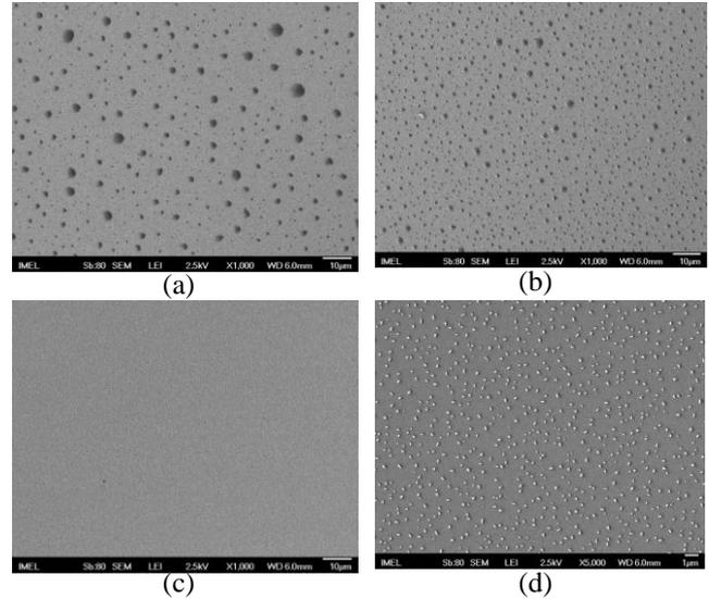
Fig. 3. SEM images (top down) of atmospheric plasma etched samples with decreasing %  $\text{O}_2$  fraction in He gas feed and after etching is finalized: (a) 1%  $\text{O}_2$  at  $t = 8$  min, (b) 0.6%  $\text{O}_2$  at  $t = 8$  min, and (c, d) pure He feed (0%  $\text{O}_2$ ) at  $t = 28$  min at two different magnifications.
