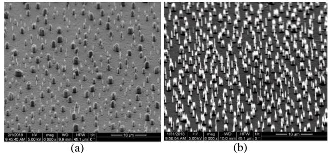
Fig. 5. SEM images of silicon pillars fabricated by atmospheric pressure plasma directed assembly followed by low-pressure plasma etching in a pulsed-gas alternating plasma process for (a) 40s and (b) 60s.
