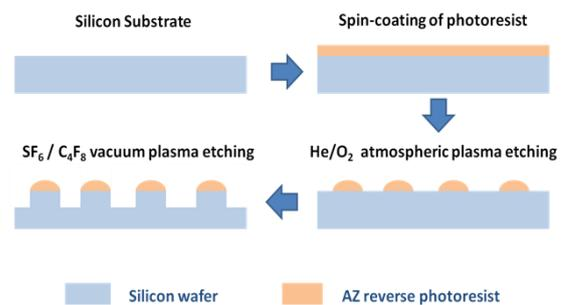
Fig. 1. Concept of atmospheric plasma directed assembly method for mask-less nanofabrication.
