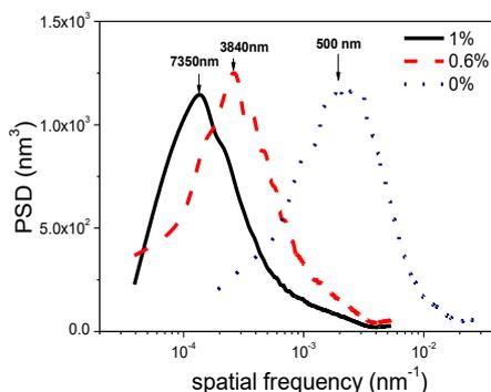
Fig. 4. Power Spectral Densities (PSD) in semi-logarithmic scales versus spatial frequency for the three contents of  $O_2$ . One can easily notice the prominent peaks demonstrating the well-defined periodicity of residues as well the dependence of their period on  $O_2$  content.
