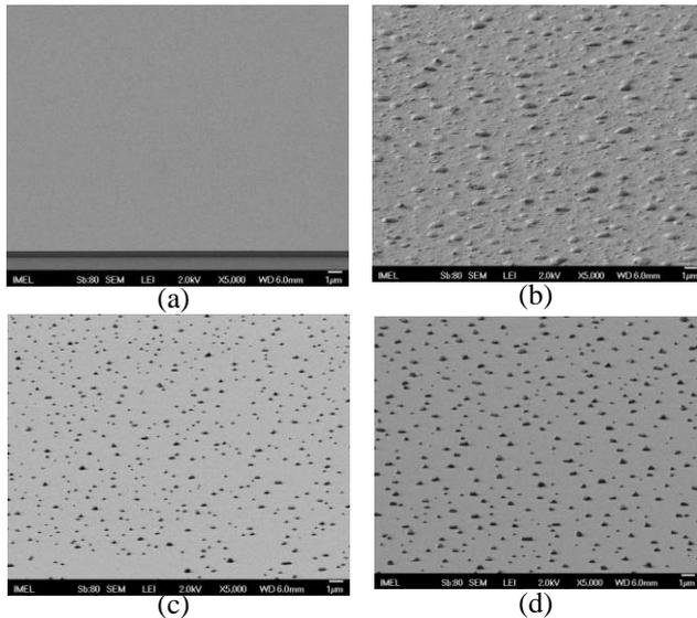
Fig. 2. SEM images ( $70^\circ$  tilt-angle) during AZ etching of Si surfaces using 0.6%  $\text{O}_2$  in He atmospheric pressure plasma in open-air condition: (a) untreated sample ( $t = 0$  min), (b)  $t = 4$  min, (c)  $t = 6$  min and (d)  $t = 8$  min.
