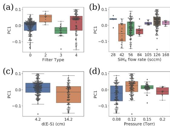
Fig. 2. Box plots showing changes of distributions regards to varying specific external parameters along PC1 obtained with SPCA. Dots represent data points. Each x-axis is (a) filter type, (b) silane flow rate, (c) distance between electrode-substrate, (d) pressure of reactor respectively.
