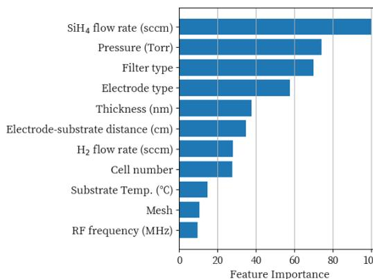
Fig. 3. Feature importance of plasma CVD of a-Si:H estimated by GBRT model.
