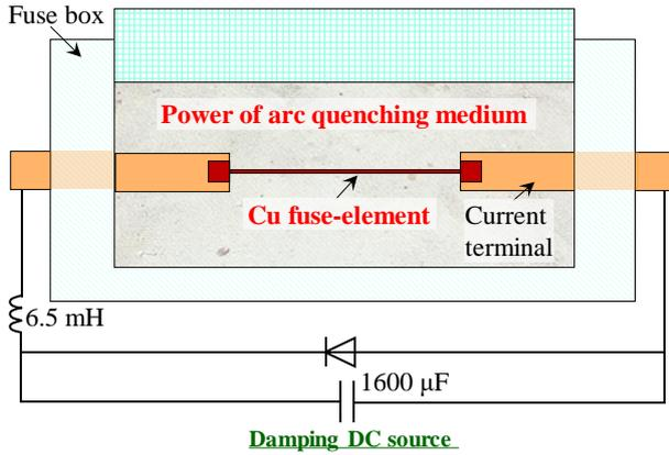
Fig. 4 Configuration of arc quenching chamber
