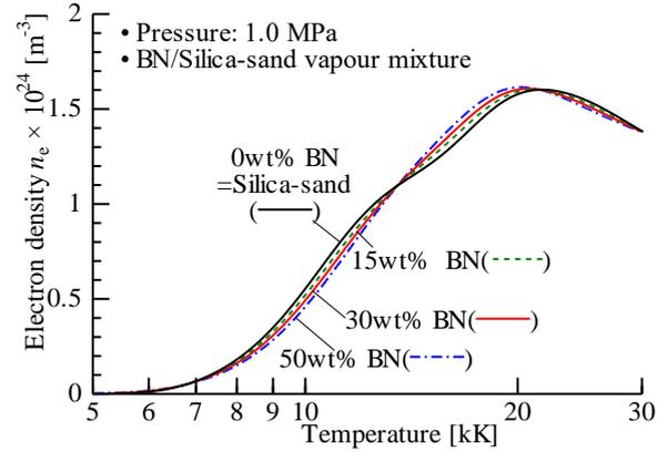
Fig.3 Electron density of BN/Silica-sand vapour mixture
