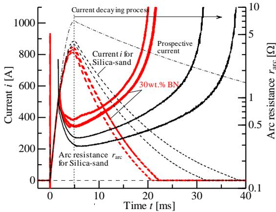
Fig.5 Current  $i$  and arc resistance  $r_{arc}$
