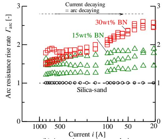
(b) Arc resistance rise rate during current decaying process
