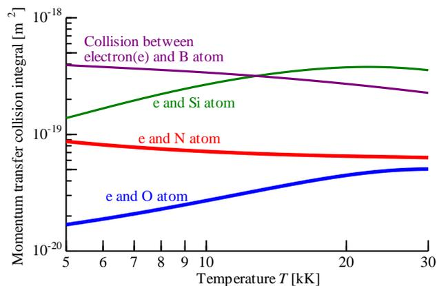
Fig.1 Electron impact collision integral of atoms
