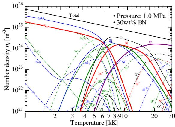
Fig.2 Number density of BN/Silica-sand vapour mixture under 30wt.% BN condition (Pressure: 1.0 MPa).
