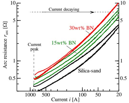
(a) Arc resistance during current decaying process
