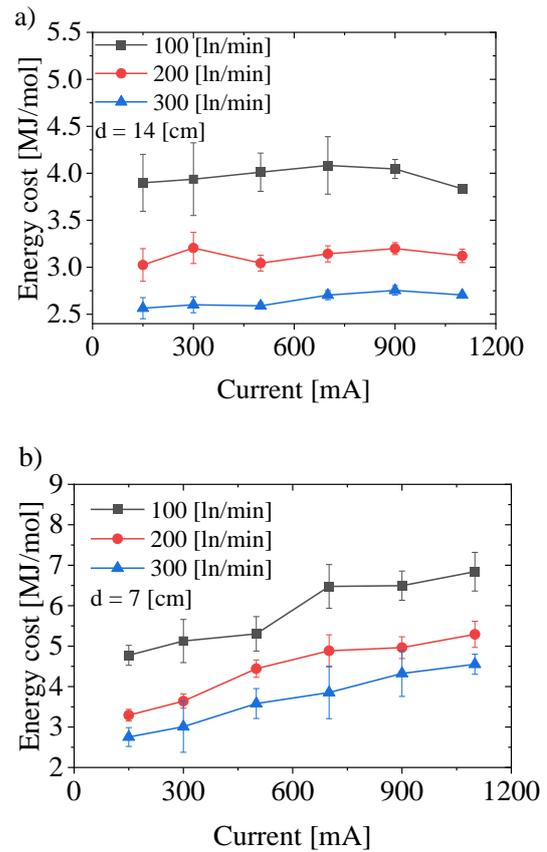
Figure 4. Energy cost as a function of the current for different flow rates, at two distances between the electrodes: a) 14 cm and b) 7cm.
