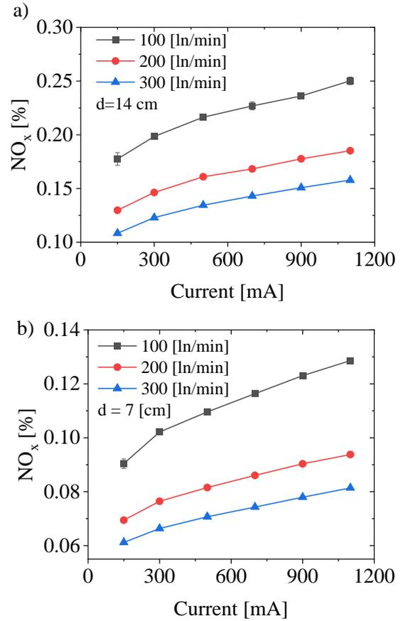
Figure 2. NO<sub>x</sub> concentration as function of the current, for different flow rates and for two distances between the electrodes: a) d = 14 cm and b) d = 7cm. Error bars are included, but are too small to be visible
