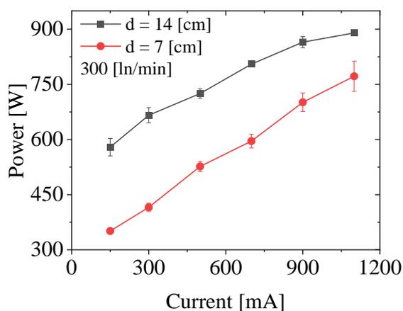
Figure 5. The power as function of current for 300 ln/min and different electrode distance. Error bars are included, but are too small to be visible for some of the points.
