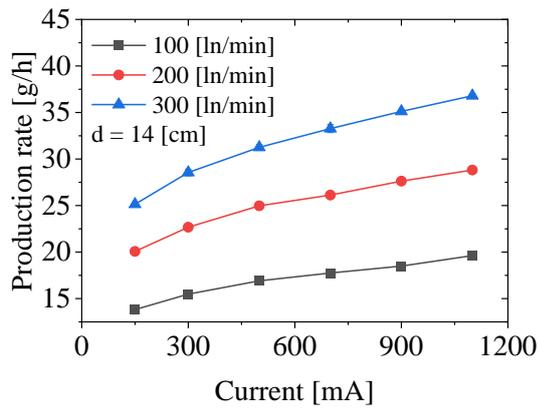
Figure 3. Production rate as function of the current for different flow rates, at a distance between the electrodes of 14 cm. Error bars are included, but are too small to be visible.
