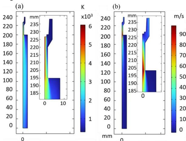
Fig. 7. Temperature (a) and velocity magnitude (b) distribution in the entire computational domain and reactor body (inset) 4 Ln/min, 0 barg and 500 mA.
