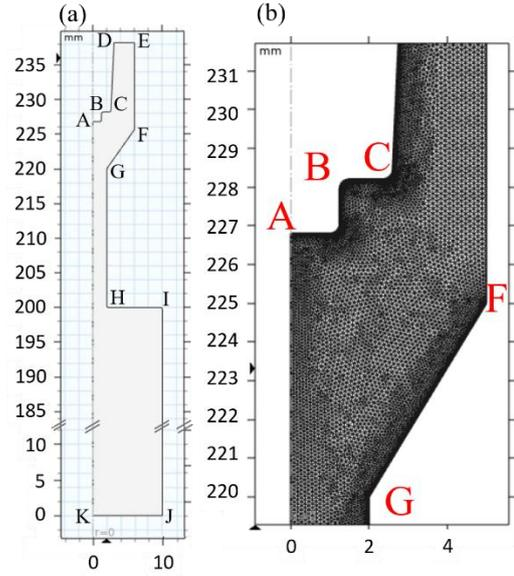
Fig. 2. 2D-axisymmetric computational domain (a) and close-up of the domain discretization (b)
