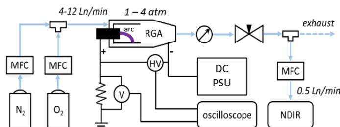
Fig. 1. Schematic representation of the RGA plasma reactor setup
