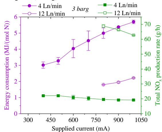
Fig. 6. Energy cost (EC) and total NO<sub>x</sub> production rate (PR) with N<sub>2</sub>:O<sub>2</sub> ratio of 1:1, as a function of the PSU current, for 4 and 12 Ln/min at an elevated pressure of 3 barg
