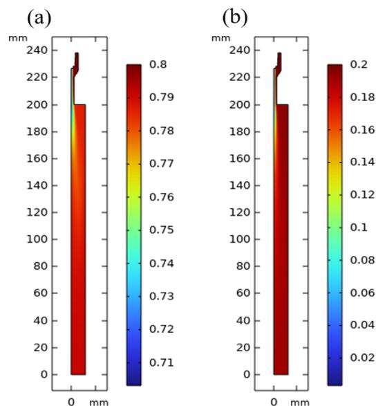
Fig. 8 Distribution plots of (a) mole fraction of  $N_2$  and (b) mole fraction of  $O_2$  in the entire computational domain for a supplied current of 500 mA, at 4 Ln/min and 0 barg.
