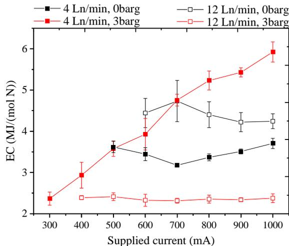
Fig. 5. Energy cost (EC) of NO<sub>x</sub> production with N<sub>2</sub>:O<sub>2</sub> ratio of 4:1, as a function of the PSU current at 4 and 12 Ln/min, and 0 barg (black) and 3 barg (red)
