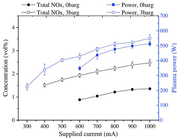
Fig. 4. Total concentration of produced NO<sub>x</sub> and plasma power with N<sub>2</sub>:O<sub>2</sub> ratio of 4:1, as a function of the PSU current at 12 Ln/min for 0 barg (whole) and 3 barg (hollow)
