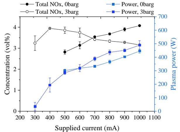
Fig. 3. Total concentration of produced NO<sub>x</sub> and plasma power with N<sub>2</sub>:O<sub>2</sub> ratio of 4:1, as a function of the PSU current at 4L/min for 0 barg (whole) and 3 barg (hollow)
