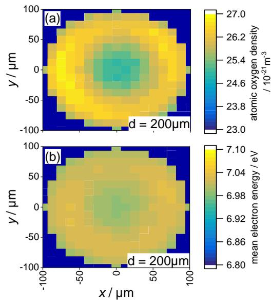
Fig. 3. 2D resolved oxygen density (a) and mean electron energy (b) for a single 200 $\mu\text{m}$  cavity [8].
