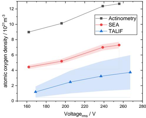
Fig. 1. Atomic oxygen density determined by various methods as a function of applied voltage [5].
