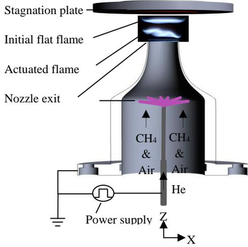
Fig. 1. Schematic representation of the burner and the plasma multi-jet devices (side view of the burner).
