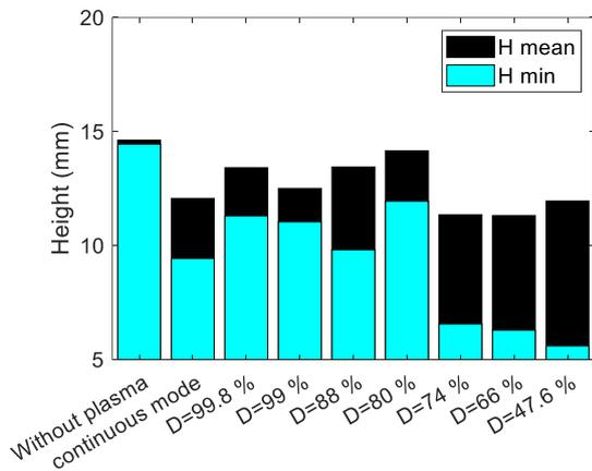
Fig. 3. Minimum flame height without plasma and with plasma (continuous mode and for different duty cycles).
