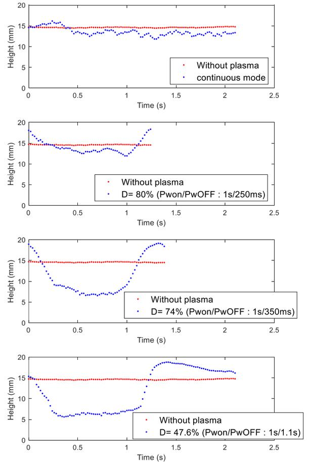
Fig. 2. Flame height without plasma (red) and with plasma (blue) at different times between consecutive pulses. (TTL cycle ON/OFF: 1s/0s (continuous mode), 1s/250ms, 1s/350ms and 1s/1.1s) (Side view of the burner).
