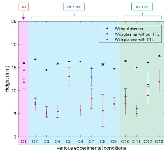
Fig. 5. Flame position without and with plasma with or without duty cycle ( $D=66\%$ ) for various experimental conditions (Fig 4).
