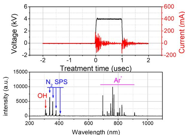
Fig. 4. The electrical (up) and optical (down) characteristics of n-PPJ
