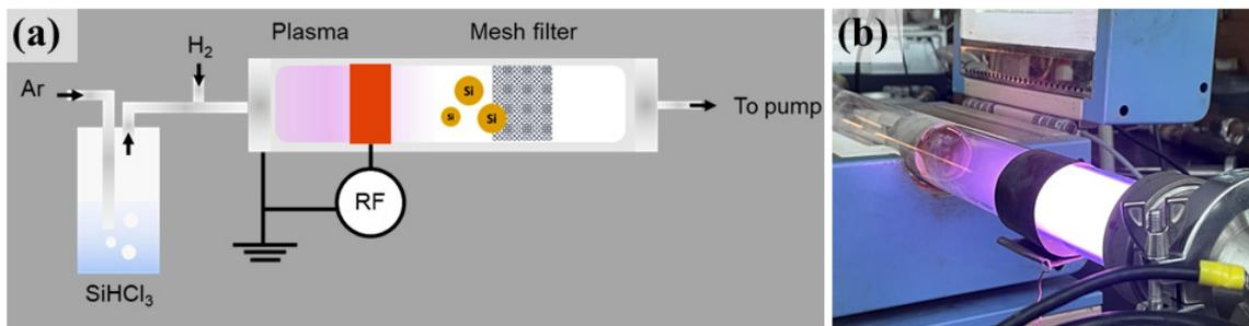
Figure 1. (a) Schematic of the precursor delivery system and of the reactor. (b) Photograph of the plasma reactor in operation.
