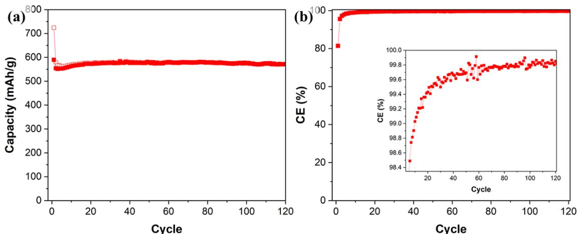
Figure 3. (a) Charge and discharge capacities for plasma-produced silicon nanoparticles. (b) Coulombic efficiency as a function of cycle number. In the inset we show the same curve in a 98.4%-100% range.
