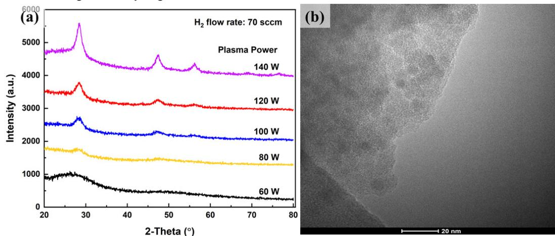
Figure 2. (a) X-ray diffraction patterns as a function of plasma input power. (b) TEM micrographs of the produced particles.
