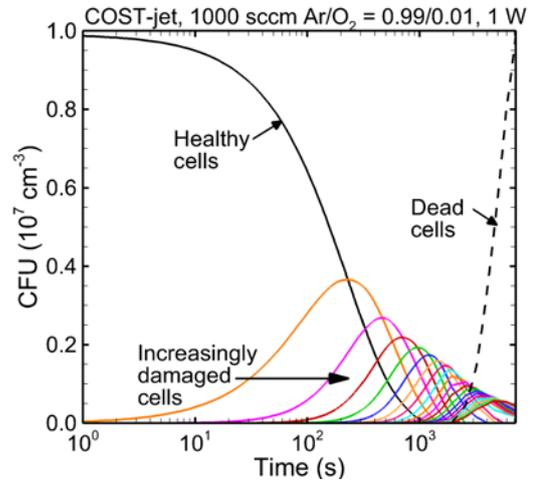
Fig. 2. Cell death for initial density of  $10^7 \text{ cm}^{-3}$  CFUs after 2 hours of treatment with Ar/O<sub>2</sub> COST-jet.
