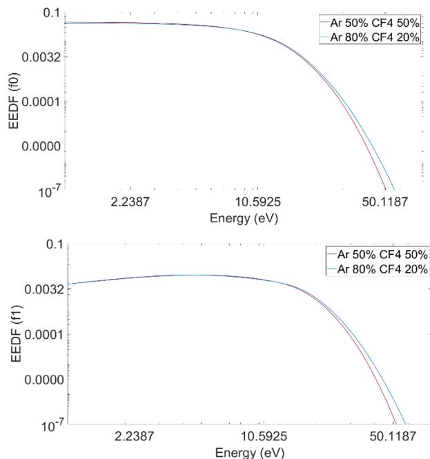
Fig. 1. Electron energy distribution functions calculated in Ar/CF<sub>4</sub> mixtures with 20% and 50% CF<sub>4</sub> at 301 Td. The EEDF is divided into (upper) the isotropic component and (lower) the anisotropic component.
