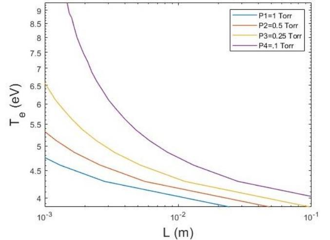
Fig. 3. The steady state electron temperature in a 1D Ar discharge from balancing bulk ionization with diffusion to the walls for various gap sizes.
