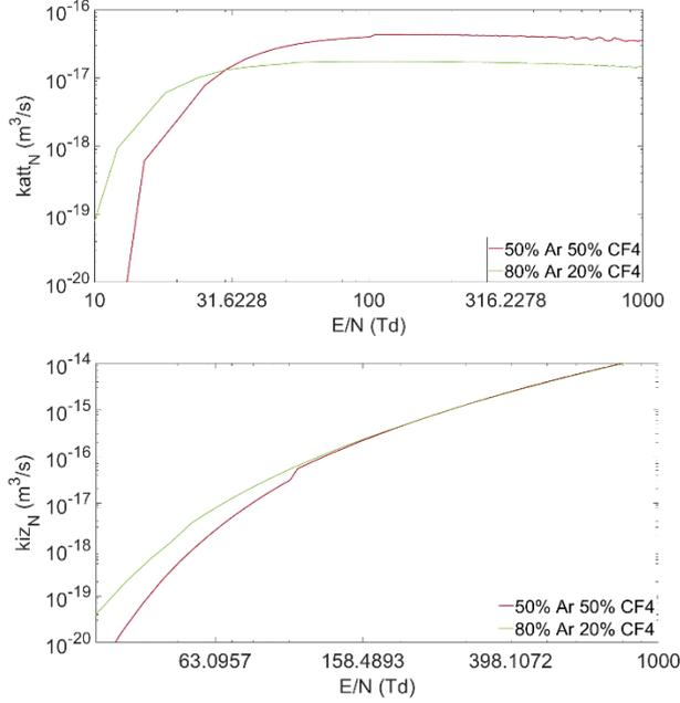
Fig. 2. Total reaction rates of electron impact processes at various reduced electric field (E/N) values. (upper)  $k_{att}$  refers to the total attachment rate and (lower)  $k_{iz}$  refers to the total ionization rate. Results are shown for 20% and 50% CF<sub>4</sub>.
