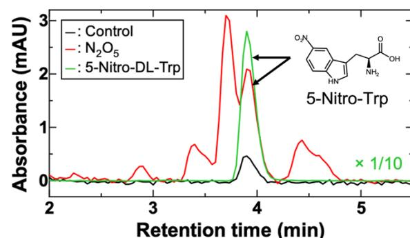
Fig. 4. LC chromatograms at 330 nm of solutions of moist tryptophan powders treated by the plasma-generated  $N_2O_5$  gas and dry air. The concentration of 5-nitro-DL-tryptophan is 100  $\mu$ M.
