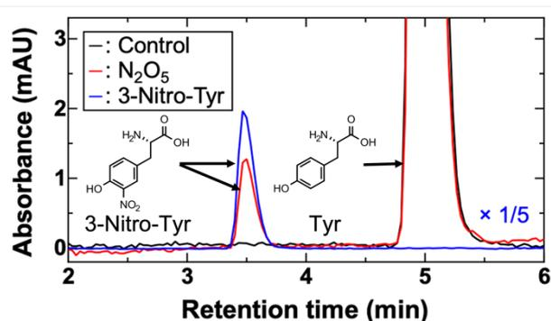
Fig. 3. LC chromatograms at 275 nm of solutions of moist tyrosine powders treated by the plasma-generated  $N_2O_5$  gas and dry air. The concentration of 3-nitro-tyrosine is 25  $\mu$ M.
