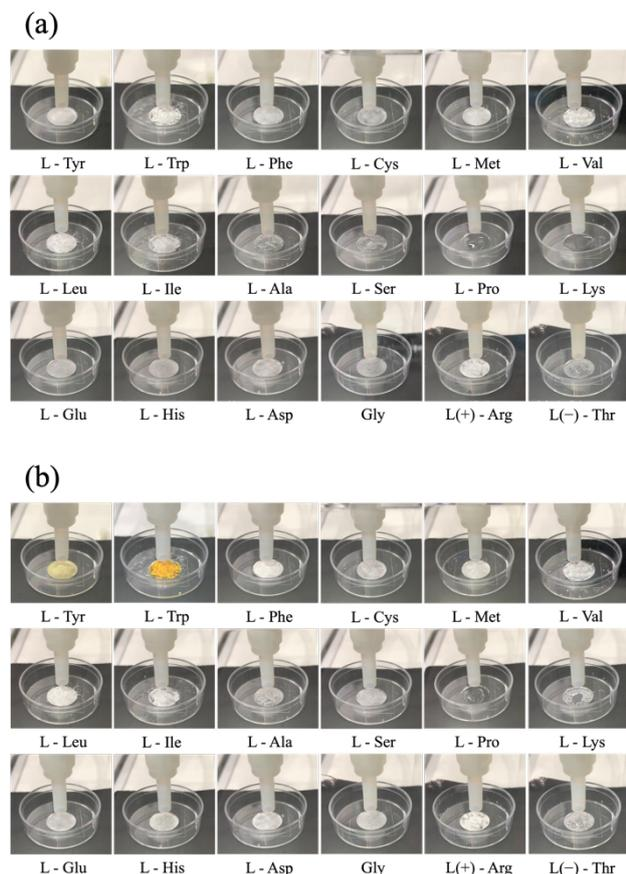
Fig. 2. Images of the moist amino acids powder (a) before and (b) after treatment of the plasma-generated  $N_2O_5$  gas for 5 min.
