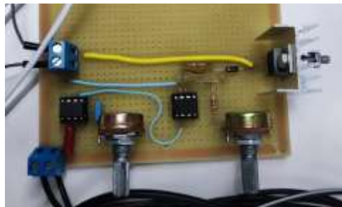
Figure 1. Electronic circuit of the prototype of the low-cost plasma pencil.
