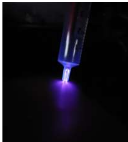
Figure 2. Corona discharge between the plasma pencil and the ground plane.
