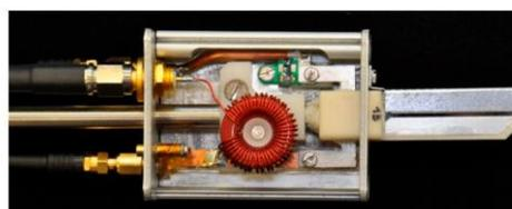
Fig. 1. Schematics (top) and a photograph (bottom) of the European Cooperation for Science and Technology (COST) plasma jet [5].
