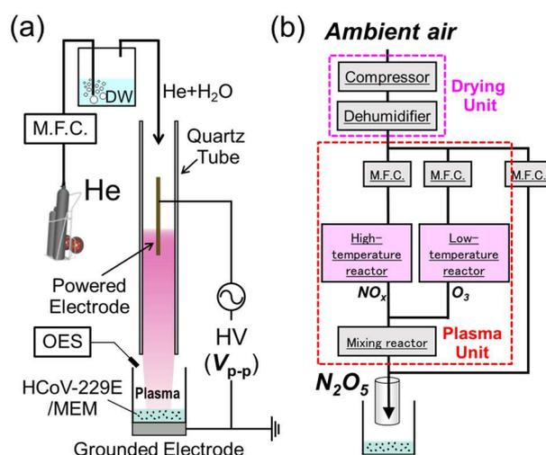
**Fig. 1.** The experimental setup for (a)  $He + H_2O$  APP exposure and (b) gaseous  $N_2O_5$  exposure to HCoV-229E virus solution.
