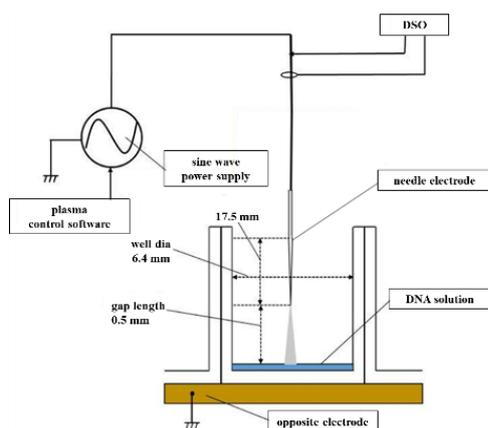
Fig. 1. Schematics diagram of plasma treatment
