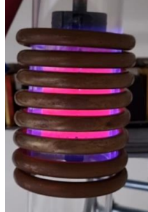
Fig. 2. Demonstration of the concept of induction-DBD hybrid reactor.
