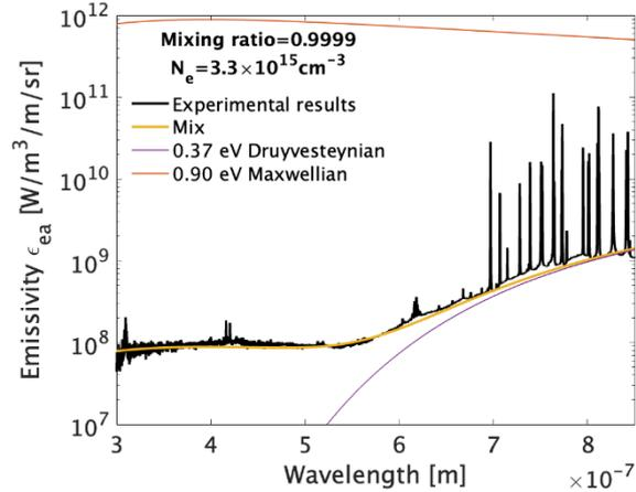
Fig. 2. Best-fitted result when discharge voltage is 5.4 kV.
