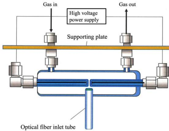
Fig. 1. Schematic diagram of this experimental setup [5].
