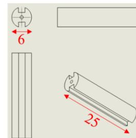
Fig. 5. Three view of two grooves electrode
