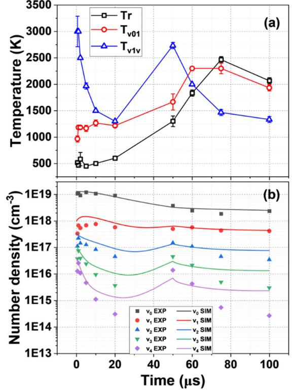
Fig. 4. (a): temperature evolution; (b): measured (scatter) and simulated (line) number density of vibrational state  $N_2(v=0-4)$ .
