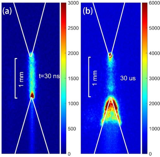
Fig. 2. (a): ICCD image of spark phase (gate width=2 ns), and (b): glow phase (gate width=2 us).
