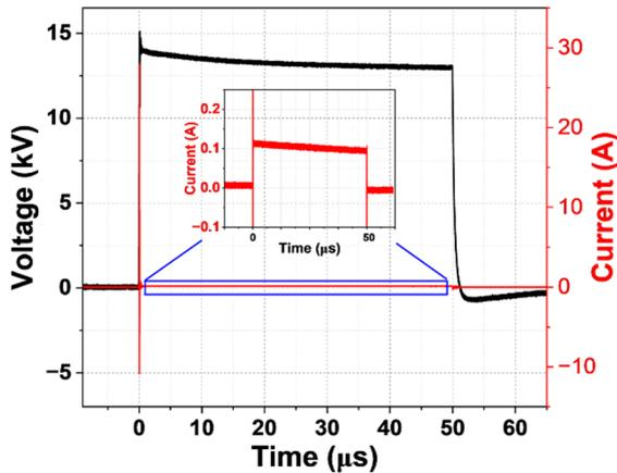
Fig. 3. Waveforms of discharge voltage and current.
