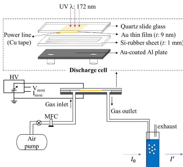
Fig. 1. Experiment set-up of photoemission-induced atmospheric pressure gas discharge.
