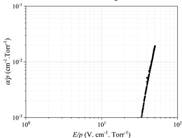
Fig. 3. Electron ionization coefficient  $\alpha/p$  as a function of the field  $E/p$  for air.
