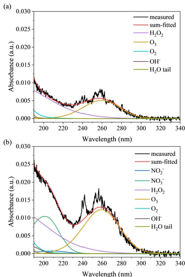
Fig. 4 Absorbance of gas discharge dissolved in water (a) excimer-irradiated gas (b) photoemission-induced air plasma
