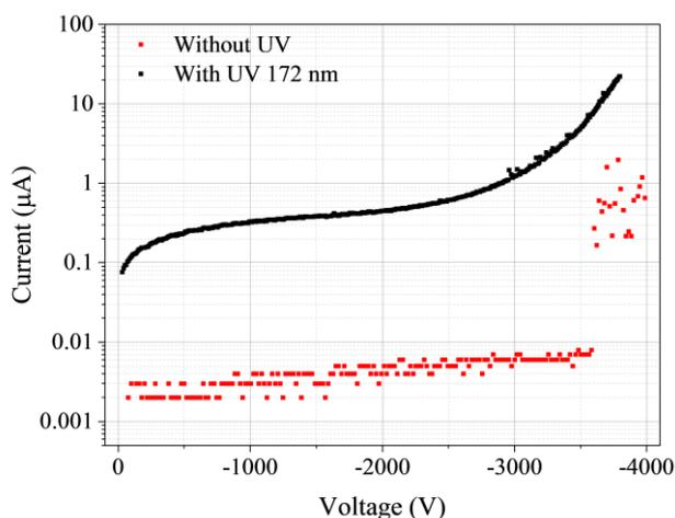
Fig. 2. Voltage-Current characteristic of photoemission-induced air discharge.
