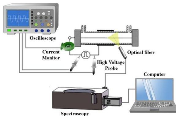
Fig. 1. Schematic diagram of DBDs experimental setup.
