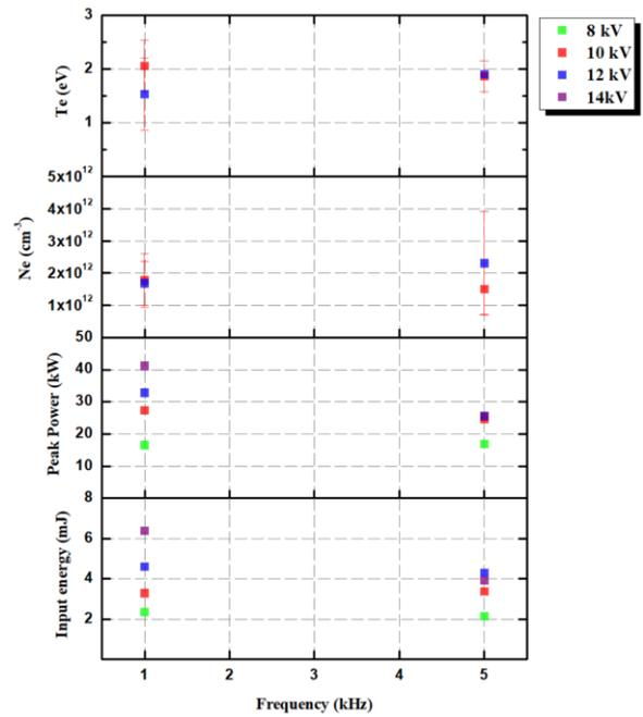
Fig. 4. Helium Plasma characteristics with a fixed pulse width of 140 ns.
