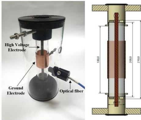
Fig. 2. Photo and diagram of DBDs reactor.
