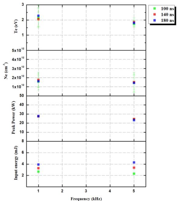
Fig. 5. Helium Plasma characteristics with a fixed applied voltage of 10 kV.
