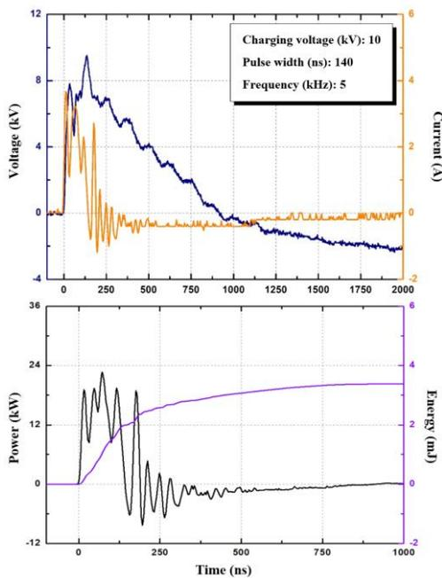
Fig. 3. Electrical diagnostics waveforms
