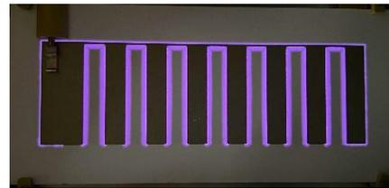
Fig. 1. Top view of SDBD, surface discharges can be seen with purple color on the  $\text{Al}_2\text{O}_3$  plate on the powered nickel electrode.
