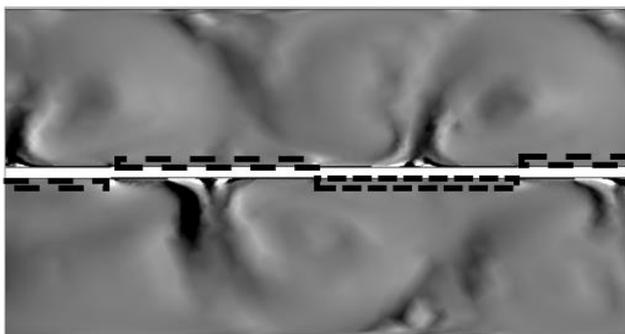
Fig. 4. 2D simulation of Schlieren effect of SDBD (black dash rectangles show the place of nickel electrodes)
