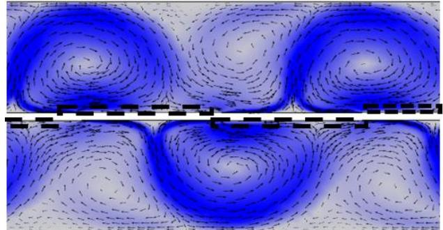
Fig. 5. 2D simulation of the velocity field of SDBD (black dash rectangles show the place of nickel electrodes)
