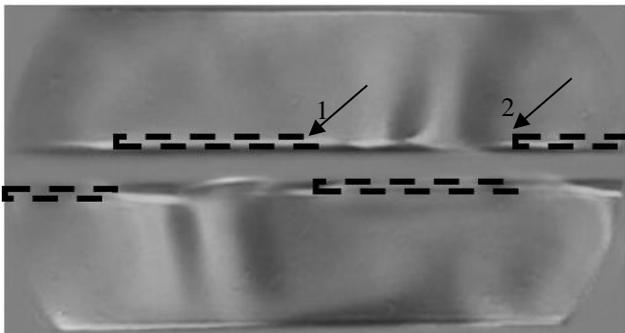
Fig. 3. Schlieren image of SDBD recorded from side window (black dash rectangles show the place of nickel electrodes in all images)
