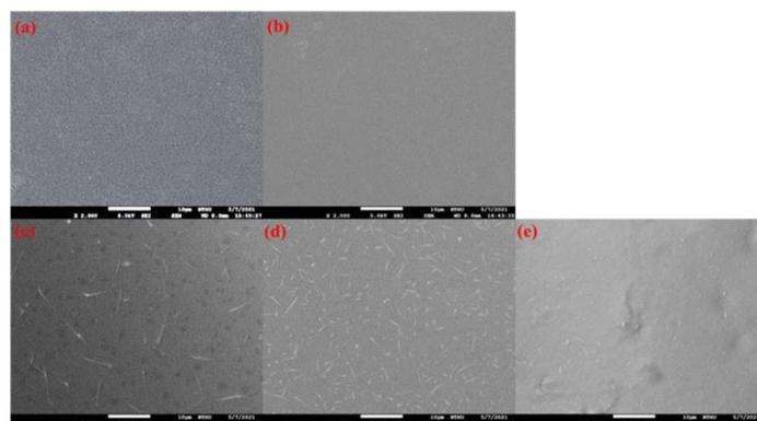
Fig.2 Surface morphologies of (a)Untreatment、(b)APPJ treatment (D:2cm/T:2min)、(c) APPJ treatment/UV-p(CA-co-DMAEMA)1:1、(d)APPJ treatment/UV-p(CA-co-DMAEMA)1:2、(e)APPJ treatment+UV-p(CA-co-DMAEMA) 2:1
