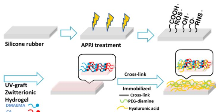
Fig.1 The schematic illustration of the preparation of functionalized surface modification with APPJ pretreatment and then graft polymerization of zwitterion hydrogels onto the silicone rubber and cross-linked HA.
