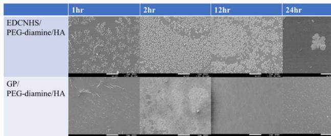
Fig.3 Surface morphologies of silicone rubber substrate after different cross-linking treatment time
