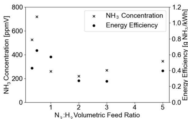
Fig. 5: Ammonia production and energy efficiency related to the feed ratio at a constant standardized flow ( $\dot{V}=60$  SCCM), constant pressure ( $p=2$   $bar_{abs}$ ), and pulse frequency ( $f=1000$  Hz). Power delivery was calculated to be 2.5  $\pm$  0.7W, depending on the conductive current.
