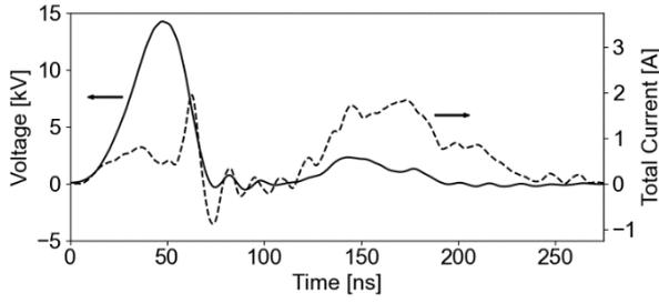
Fig. 2: Pulse characterization of the nanosecond pulser and corresponding current discharge of a 1:1 N<sub>2</sub>:H<sub>2</sub> gas mixture at  $p=3$  bar<sub>abs</sub> and  $d=2$  mm.
