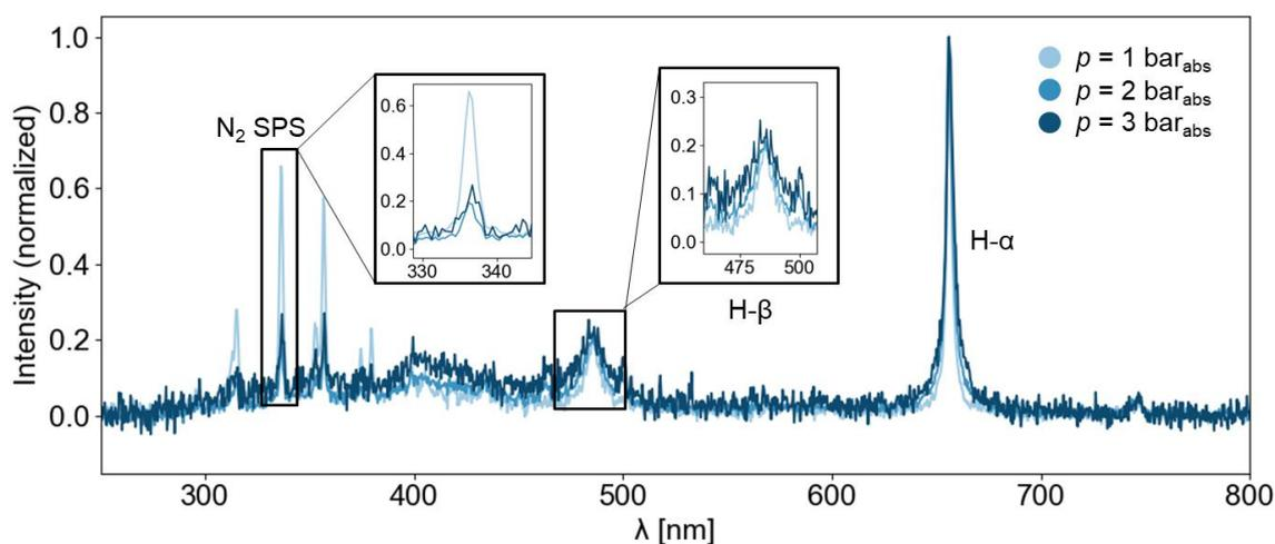
Fig. 4: Emission spectra of a plasma discharge sustained at various pressures at a set pulse frequency ( $f=1000$  Hz) and  $N_2:H_2$  feed ratio (1:1).
