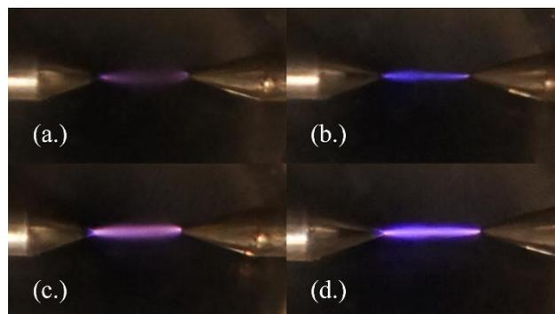
Fig. 1: Images of the plasma formed between two pin electrodes at atmospheric pressure ( $p=1$  bar<sub>abs</sub>). The diffuse 1:1 N<sub>2</sub>:H<sub>2</sub> mixture (a.) and pure N<sub>2</sub> (b.) plasmas were produced at lower voltages than the sparking 1:1 N<sub>2</sub>:H<sub>2</sub> mixture (c.) and pure N<sub>2</sub> (d.) plasmas.
