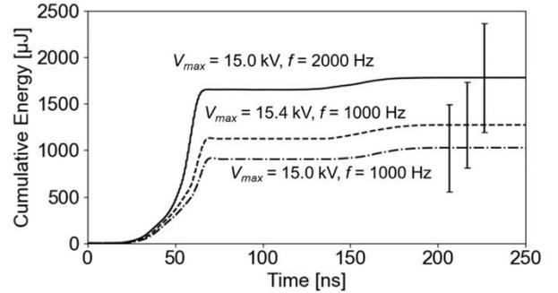
Fig. 3: Cumulative energy per pulse delivered to the plasma from the nanosecond pulser with a 1:1 N<sub>2</sub>:H<sub>2</sub> ratio gas flow at  $p=2.5$  bar<sub>abs</sub> and  $d=2$  mm.
