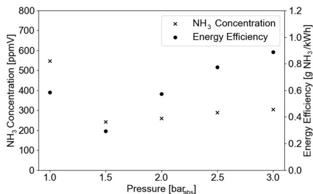
Fig. 6: Ammonia production and energy efficiency at various pressure with a constant standardized flow ( $\dot{V}=60$  SCCM),  $N_2:H_2$  volume feed ratio (1:1), and pulse frequency ( $f=1000$  Hz). Power was scaled to reach breakdown conditions.
