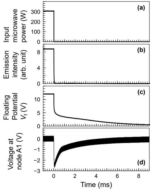
Fig. 4. Temporal changes of (a) input microwave power, (b) emission intensity, (c) floating potential  $V_f$ , and (d) voltage at node A1 measured in afterglow phase of surface-wave plasma, with the conventional FHP system and the  $V_f$ -monitoring probe shown in Fig. 2(a).
