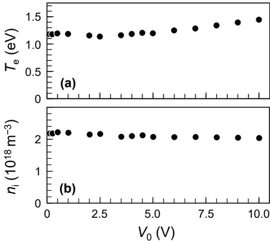
Fig. 3. (a) Electron temperatures  $T_e$  and (b) ion densities  $n_i$  measured by the conventional FHP method with various  $V_0$  values. Discharge conditions were at Ar, 10 Pa, 300 W.
