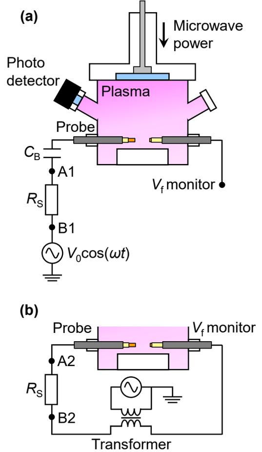
Fig. 2. Schematic diagrams of (a) conventional FHP measurement system and (b) modified FHP measurement system developed in this study.
