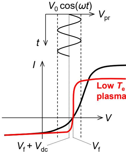
Fig. 1. Schematic of a relationship between the applied AC voltage in the FHP method and the  $I-V$  curve measured in the LP method. The red line shows an  $I-V$  curve of low  $T_e$  plasma (e.g. afterglow) considered in this study.
