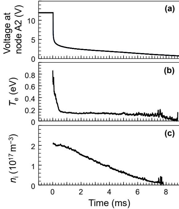
Fig. 5. Temporal changes of (a) voltage at node A2, (b) electron temperature  $T_e$ , and (c) ion density  $n_i$  measured in afterglow phase of surface-wave plasma, with the modified FHP system shown in Fig. 2(b).
