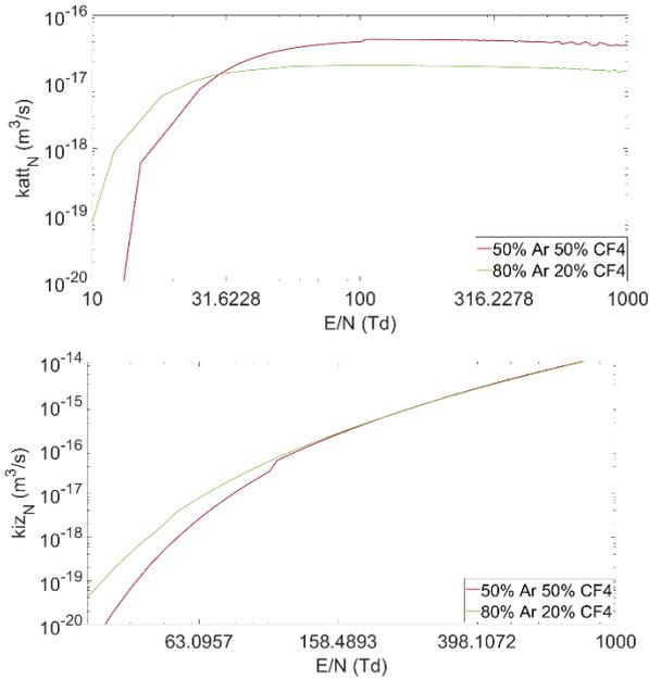
Fig. 4. Reaction rates of electron impact processes at various reduced electric field ( $E/N$ ) values. (upper)  $k_{att}$  refers to attachment and (lower)  $k_{iz}$  refers to ionization. Results are shown for 20% and 50% CF<sub>4</sub>.
