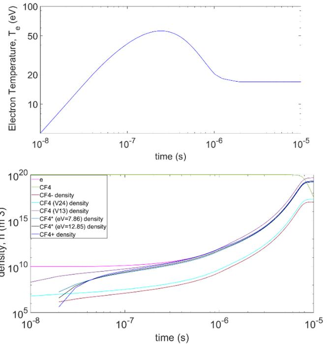
Fig. 5. (upper) Electron temperature vs time, and (lower) the density for all gas species in Table 1. The system is 100% CF<sub>4</sub> and includes only electron-impact reactions.
