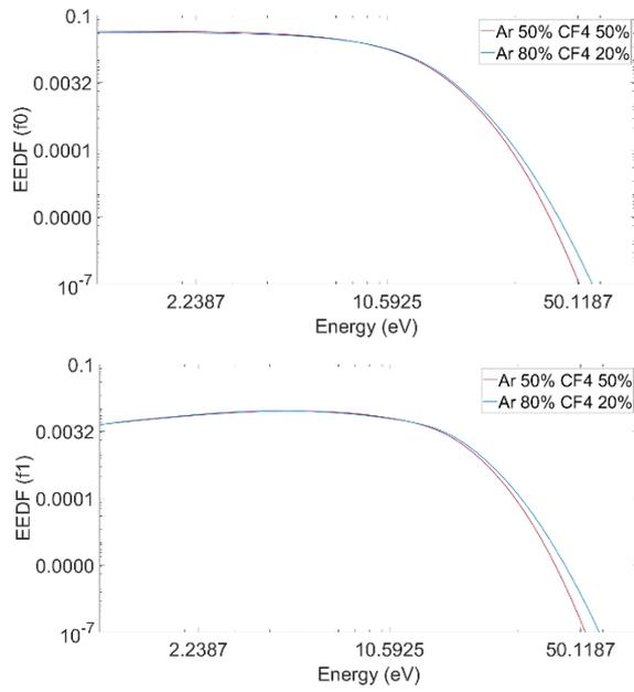
Fig. 3. Electron energy distribution functions calculated in Ar/CF<sub>4</sub> mixtures with 20% and 50% CF<sub>4</sub> at 301 Td. The EEDF is divided into (upper) the isotropic component and (lower) the anisotropic component.
