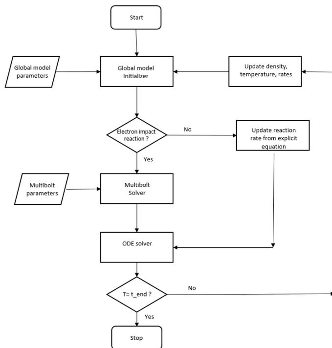
Fig. 1. Flow chart of the global model coupled with Multibolt.
