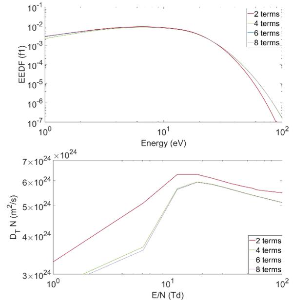
Fig. 2. (upper) The anisotropic component of the electron energy distribution EEDF when considering a different number of terms in the spherical harmonic expansion with a reduced electric field of 1000 Td. (lower) The transverse diffusion coefficient for varying values of reduced electric field (E/N) for Ar/CF<sub>4</sub> = 80/20.
