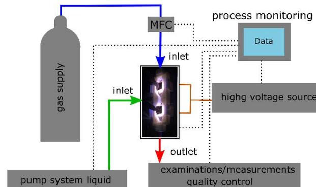
Fig. 4. Experimental schematic diagram of the ZPPK reactor system for the treatment of a liquid with various gases
