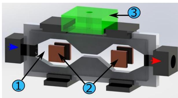
Fig. 3. ZPPK reactor: blue arrow: inlet (process gas); red arrow: outlet; (1) first reactor chamber; (2) square electrodes; (3) inlet/access (liquid).
