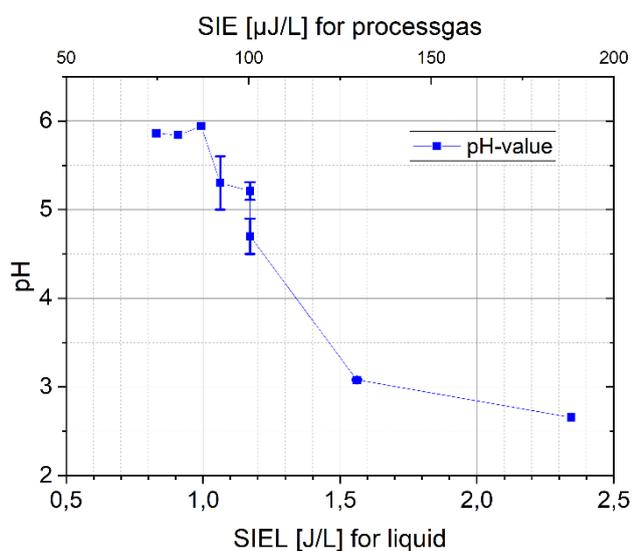
Fig. 6. pH value of the treated water as a function of SIE [ $\mu\text{J/L}$ ] and SIEL [ $\text{J/L}$ ]
