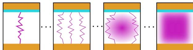
Fig. 2. Classification of usable plasma states: filamentary plasma on the left and homogeneous/diffuse plasma on the right. [6, 7]
