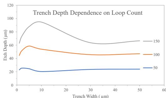
Fig. 3 Trench etch depths with increasing loop counts of 50, 100 and 150.
