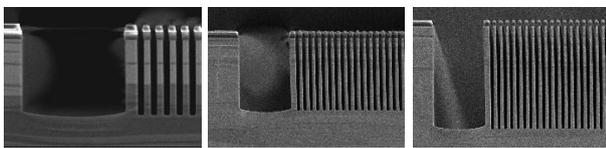
Fig. 2 ARDE compensated etching of 1.5 and 30  $\mu\text{m}$  trenches at 50 (left), 100 (middle) and 150 (right) loops.
