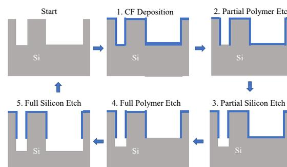
Fig. 1 Schematic illustration of a five step Bosch loop process to etch a wide and narrow trench with different AR.
