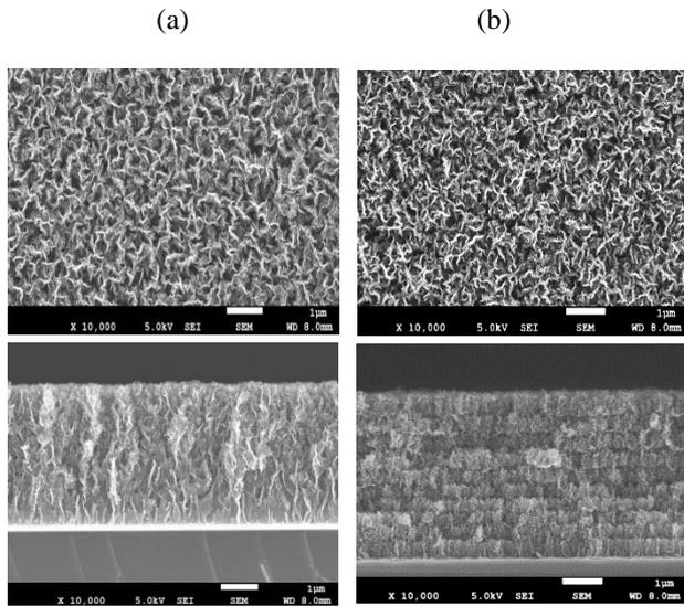
Fig.3. SEM top surface and cross-section images of CNW deposited (a) without plasma treatment with 60s deposition time and (b) inter-synthesis cyclic plasma treatment method with 12 cycles (each cycle: CNW synthesis for 5s, plasma treatment for 5s)
