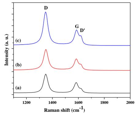
Fig.4. Raman spectra of CNW films (a) without any plasma treatment with 60s deposition time (b) post plasma treatment with 10s  $O_2/Ar:0.1/10sccm$  plasma, and (c) CNW prepared by inter-synthesis cyclic plasma treatment method with 12 cycles (each cycle: CNW synthesis for 5s, plasma treatment for 5s)
