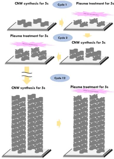
Fig.2. Schematic representation of depositing CNW by cyclic operation of PECVD and plasma treatment (1 cycle: CNW synthesis for 5s, plasma treatment for 5s).
