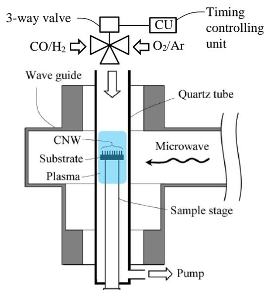
Fig.1. Schematic representation of MPECVD system
