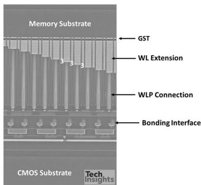
Fig. 1. Example of bonding process (YMTC 64-layer 3D Xtacking in Nand Flash) [3]
