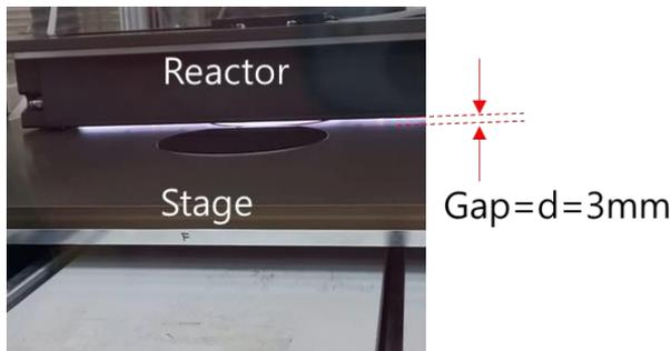
Fig. 3. Atmospheric plasma treatment side view
