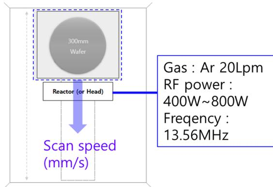
Fig. 2. Ar Atmospheric plasma Schematics
