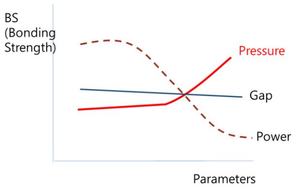
Fig. 6. Parameter vs Bonding Strength (abs)
