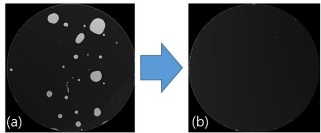
Fig. 4. SAT images: (a) Bulk voids affected by particles during bonding, and (b) Suppressed voiding by partition
