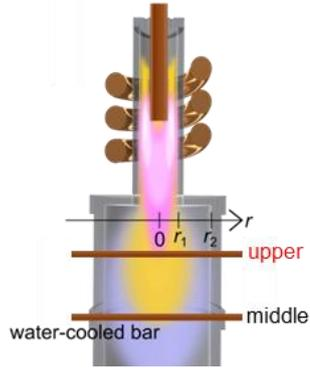
Figure 1. Schematic illustration of the geometry of the thermal plasma chamber with a water-cooled copper bar placed at the position near(upper) and far(middle) from the plasma.
