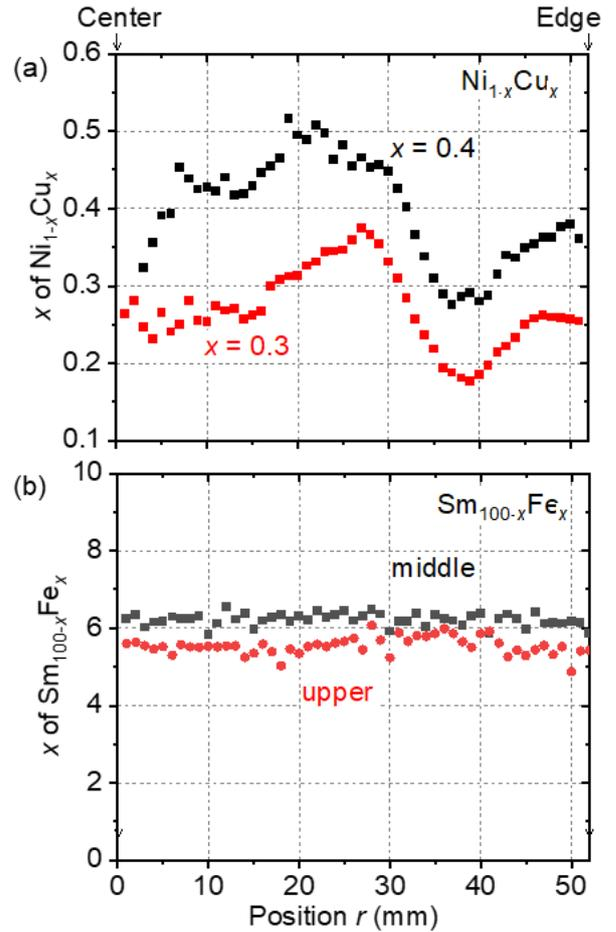
Figure 2 Cu and Sm concentration as a function of the radial position,  $r$ , from the center ( $r = 0$  mm) to the edge of the chamber for (a)  $\text{Ni}_{0.7}\text{Cu}_{0.3}$  and  $\text{Ni}_{0.6}\text{Cu}_{0.4}$  and (b)  $\text{Sm}_7\text{Fe}_{93}$  nanopowders. For Ni-Cu case, the position of the bar was middle. Reproduced by permission from[6], copyright [2023, Elsevier] for (a).
