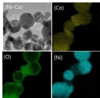
Fig. 2. FE-TEM and EDS image of Ni-Co.
