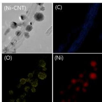
Fig. 3. FE-TEM and EDS image of Ni-CNT.
