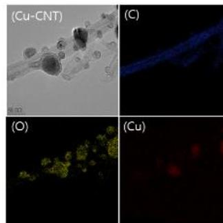
Fig. 4. FE-TEM and EDS image of Cu-CNT.
