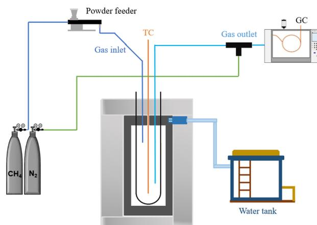
Fig. 1. Schematic diagram of electric furnace for methane pyrolysis.
